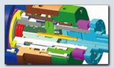
Floating cylinder design of tool clamp/unclamp system eliminates unnecessary force on the spindle bearings during tool change and prolongs spindle bearing life.
