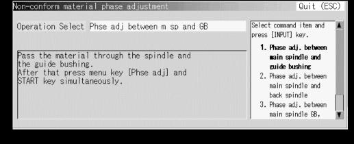
Lastly, add M26 to bar loader sub program to line up guide bushing and main spindle at bar change.
